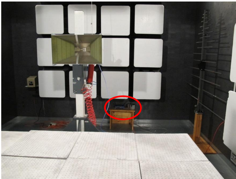
Fig. 3.1 Wi-Fi router is placed within the red circle
